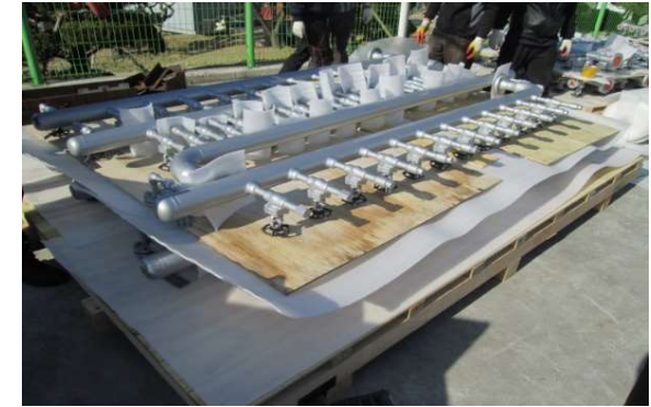
steam manifold completed
