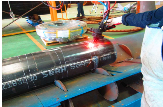
fabrication in process: LPG cutting
