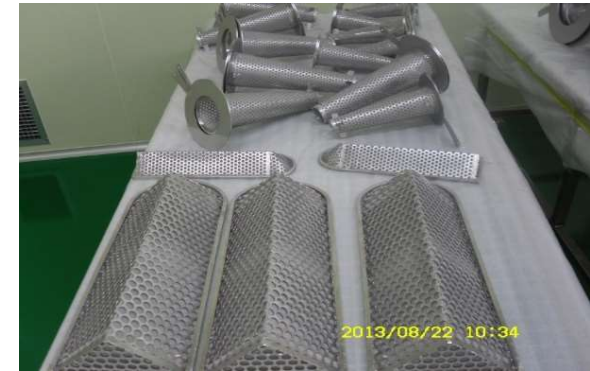
straining units: perforated plate and meshed screen
