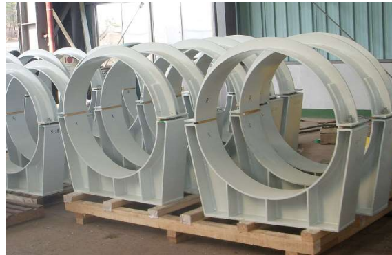
pipe support structures
