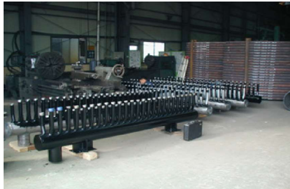
lower boiler header
