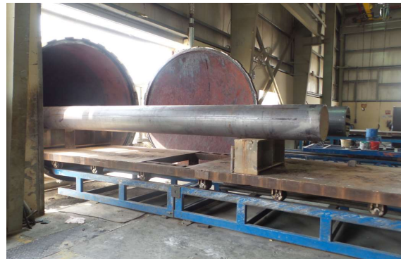
autoclave curing of rubber lined pipes
