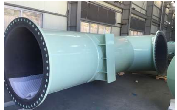
completion of rubber lining
